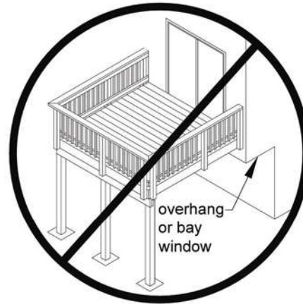
Figure 18. No Attachment to House Overhang with Ledger.
